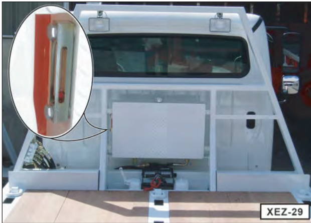
Figure 8-1. Sight Glass On Hydraulic Oil reservoir.
