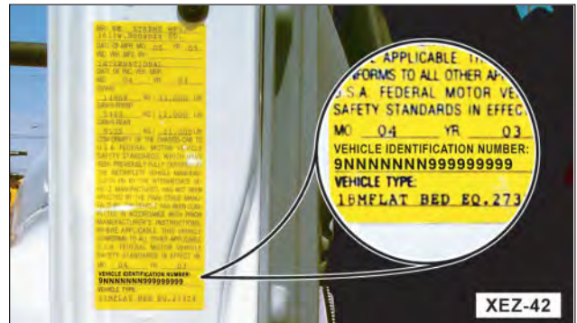
Figure 1-4. Vehicle Identification Number (VIN).
