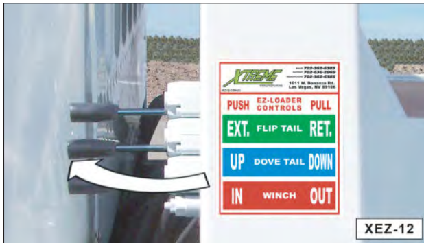
Figure 7-10. Push Dove Tail Control Lever To The UP Position.
