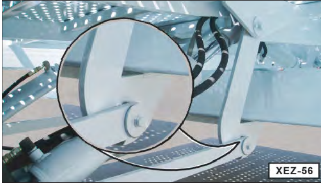
Figure 7-31. Make Sure Flip Tail Engages Locking Mechanism.
