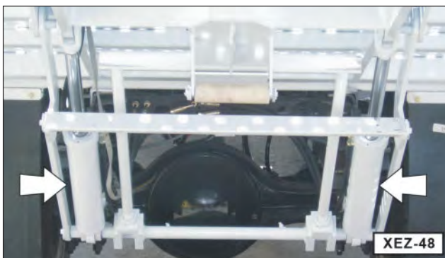
Figure 6-8. Dove Tail Hydraulic Cylinders.
