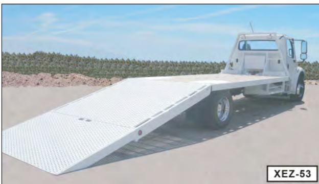
Figure 7-18. Make Sure Ramp Is Firmly Grounded.
