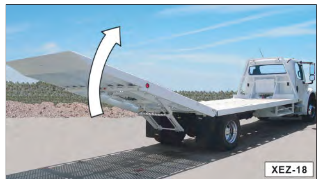
Figure 7-15. Make Sure The Ramp (Dove And Flip Tail) Is Fully Extended.
