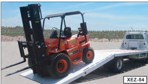
Figure 7-21. Place Load On EZ Loader. For information call (800) 497-1704
