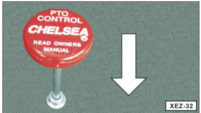
Figure 7-35. Disengage Power Take Off.
