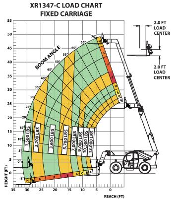
LOAD RATINGS ARE FOR VEHICLE EQUIPPED WITH FOAM FILLED OR SOLID TIRES. LOAD INCLUDES WEIGHT OF ANY RIGGING 6,500 LBS AT 24 IN MIN CAPACITY FORK (13,000 LBS PAIR)
