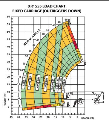
THE REAR AXLE MUST BE LOCKED AND THE OUTRIGGERS FIRMLY AGAINST THE GROUND. LOAD RATINGS SHOWN ARE FOR VEHICLES EQUIPPED WITH FOAM FILLED OR SOLID TIRES ONLY LOAD INCLUDES WEIGHT OF RIGGING 7,500 LBS AT 24 IN MIN CAPACITY FORK (15,000 LBS PAIR).
