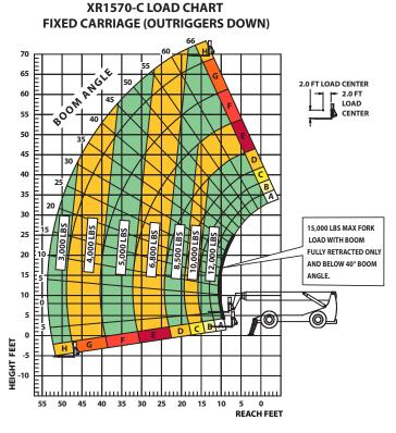
THE REAR AXLE MUST BE LOCKED AND THE OUTRIGGERS FIRMLY AGAINST THE GROUND. LOAD RATINGS SHOWN ARE FOR VEHICLES EQUIPPED WITH FOAM FILLED TIRES ONLY. 7,500 LBS AT 24<sup>°</sup> MIN CAPACITY FORK (15,000 LBS PAIR).
