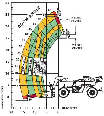
LOAD RATINGS SHOWN ARE FOR VEHICLES EQUIPPED WITH FOAM FILLED TIRES ONLY.
