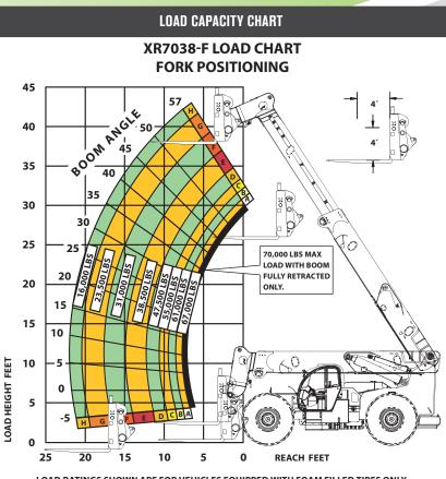
LOAD RATINGS SHOWN ARE FOR VEHICLES EQUIPPED WITH FOAM FILLED TIRES ONLY. 35,000 LBS AT 24<sup>°°</sup> MIN CAPACITY FORK (70,000 LBS PAIR).
