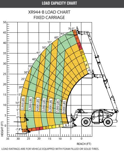
LOAD INCLUDES WEIGHT OF ANY RIGGING
