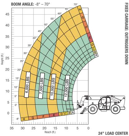
Rear axle must be locked and outriggers firmly against ground. Load ratings shown are for vehicles equipped with foam-filled or solid tires. Load includes weight of any rigging. 6,000 lbs. at 24" minimum capacity/fork (12,000 lbs./pair).
